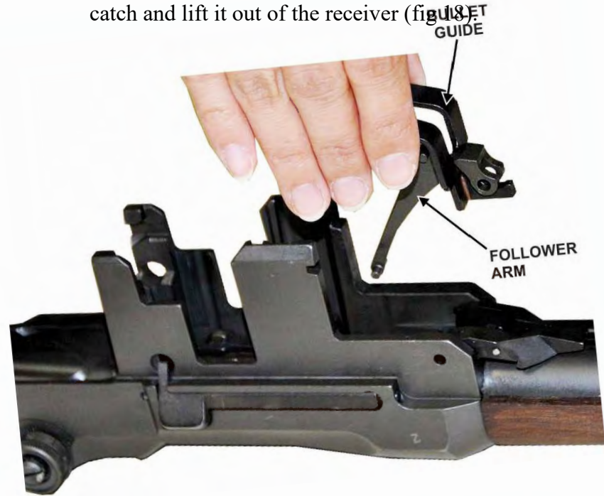
Figure 17. Bullet guide and follower arm removal
