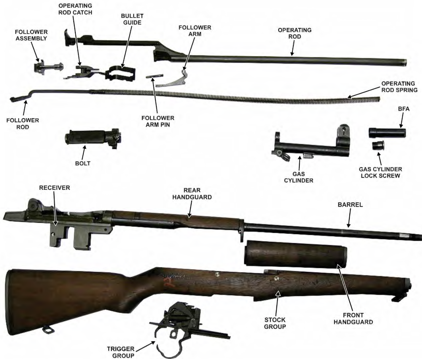
Figure 29. Disassembled parts of M1 Garand Rifle
