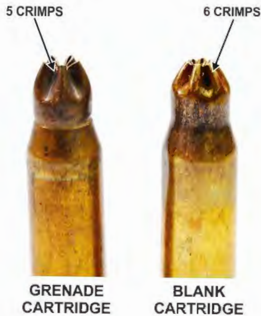
Figure 87. Grenade Cartridge vs. Blank Cartridge
