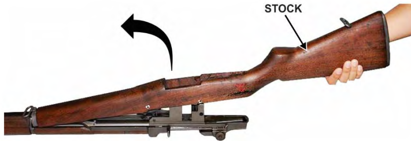
Figure 13. Lifting up stock
