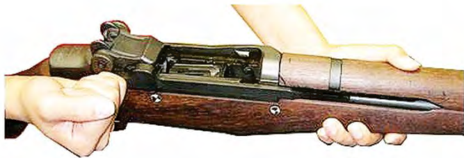
Figure 1. Pulling operating rod
