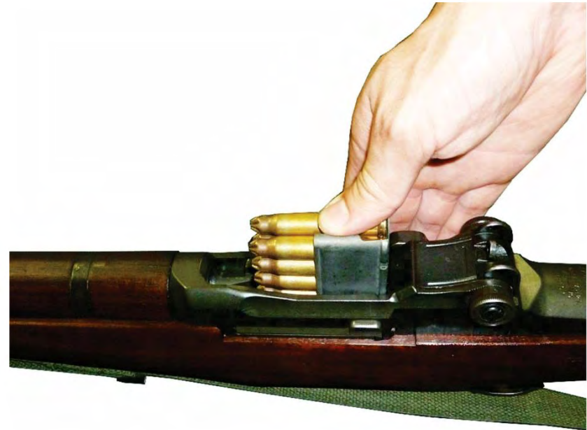
Figure 56. Loading of clip into rifle
