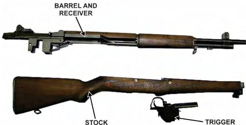
Figure 7. Trigger group, barrel and receiver group, and stock group
