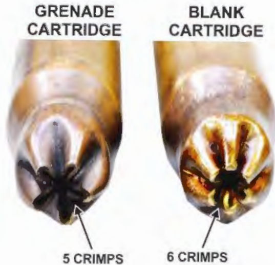
Figure 88. Grenade Cartridge vs. Blank Cartridge
