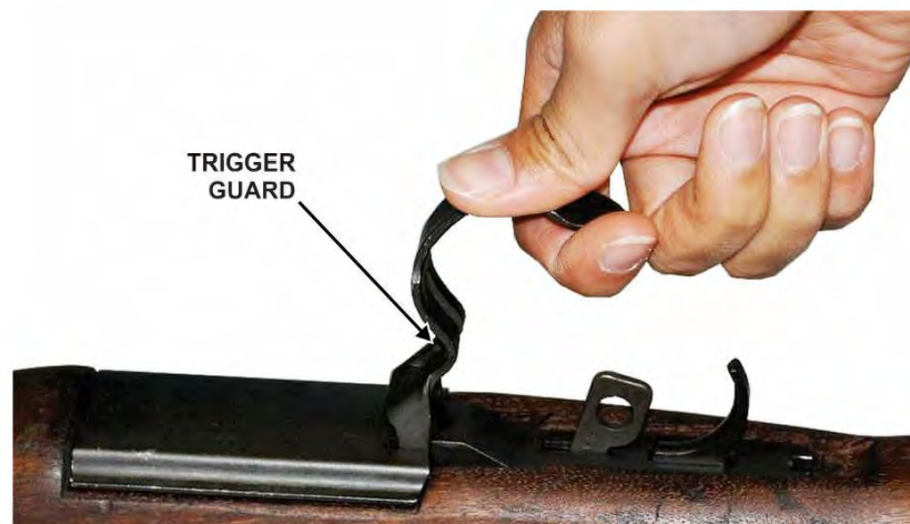
Figure 11. Trigger guard being pulled rearward and upward
