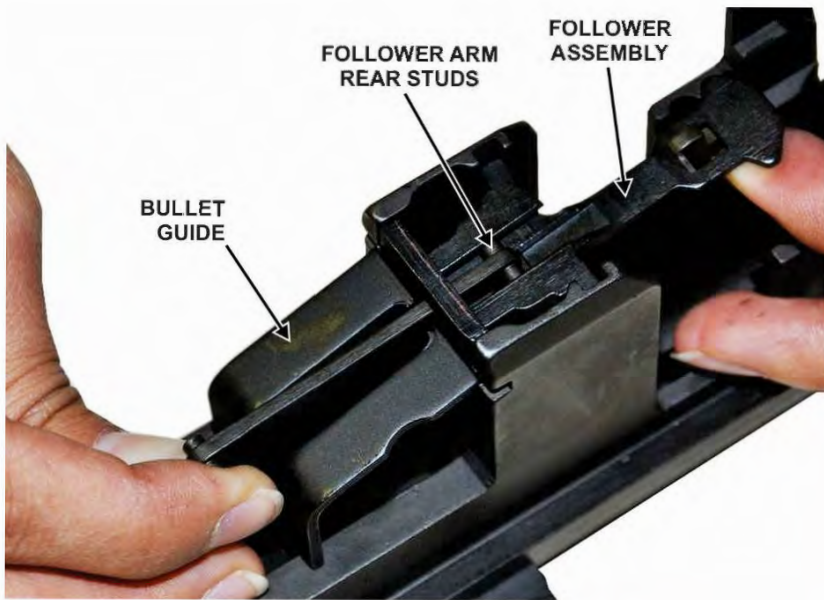
Figure 47. Installing follower arm
