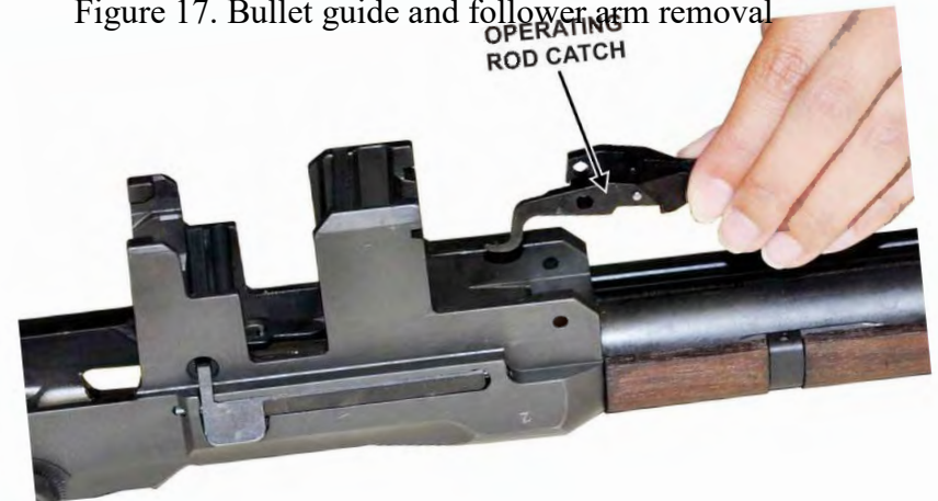
Figure 18. Operating rod catch removal
