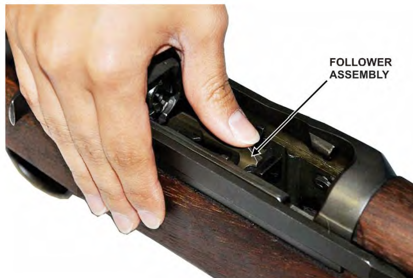
Figure 9. Depressing the follower assembly
