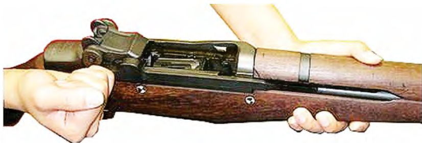
Figure 8. Checking that weapon is clear
