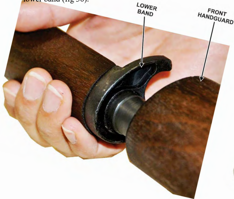
Figure 30. Front hand guard insertion
