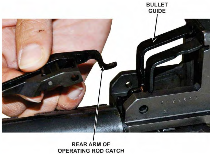
Figure 43. Rear arm of operating rod catch
